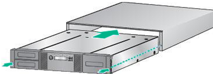
Figure 5: Installing the tabletop conversion cover
