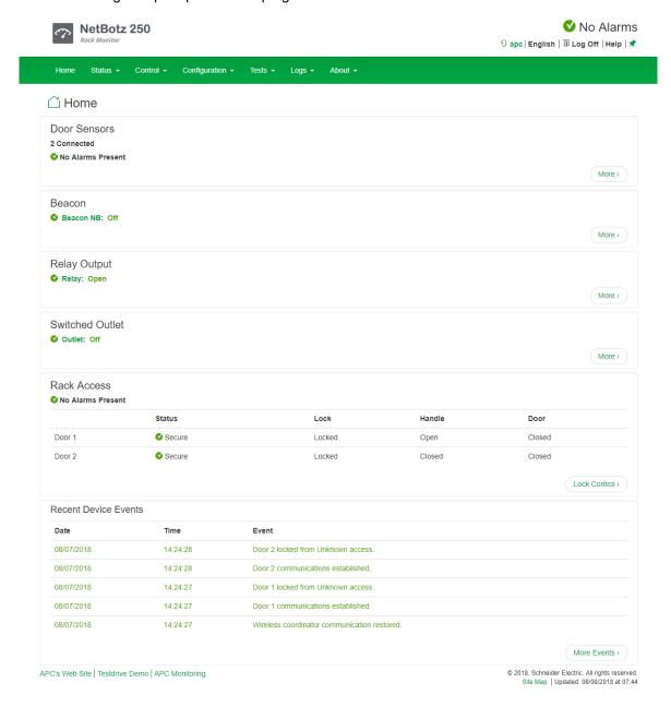
The **Home** tab displays the alarm status of system devices: Critical (device requires immediate attention), Warning (attention required), or Normal (no alarms).
